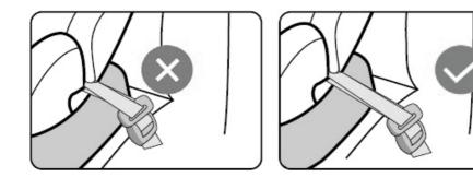
IMPORTANT! The 3-point vehicle belt must not touch the car seat!
