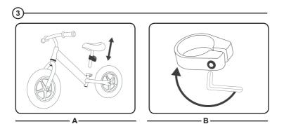
**CAUTION!** Adjust the height of the saddle by following the security tag on the post (the mark must not be visible).
